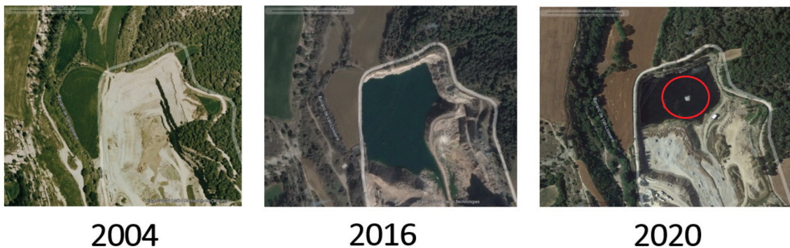
Figure 7.1.3.3. Satellite images of the Fitó quarry in different years. The red circle in the image corresponding to 2020 shows where the plastic insulation came free.
